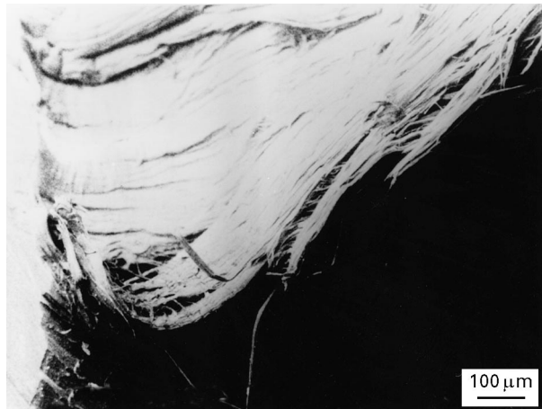
Figure 4 A higher magnification view of band C showing the highly drawn fibres with their ends pulled out of the material matrix.
